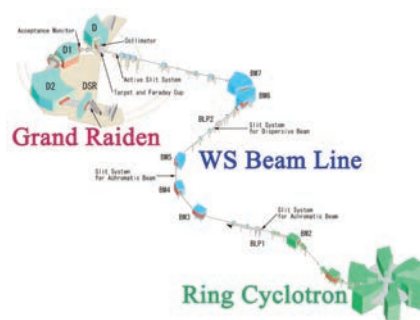
図 1.21: A schematic view of the high energy-resolution facility of RCNP, Osaka, consisting of the RCNP Ring cyclotron, a high-dispersion beam line “WS course” and a high-resolution magnetic spectrometer “Grand Raiden”.
